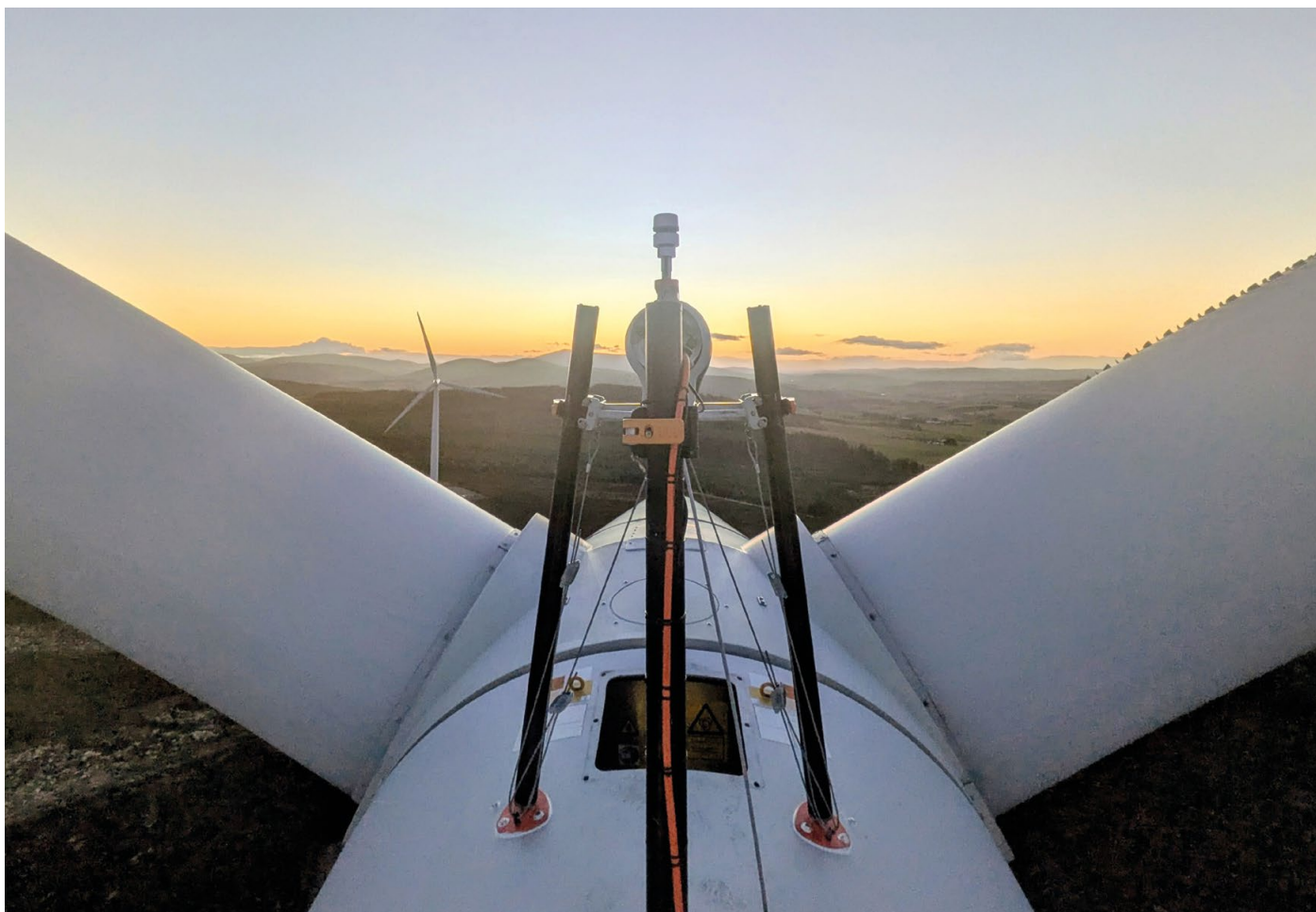
Dynamic Yaw measurement system upgrade at Hill of Towie (Credit: ZX Measurement Services).
